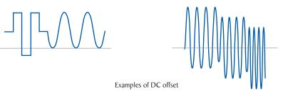
The 9830 Series is capable of generating AC+DC waveforms. When operating in pulse, step and list mode, the AC signal can be combined with either a positive or negative DC offset voltage, allowing users to create a wide range of waveforms.
